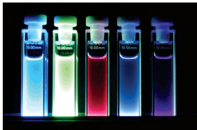
Figure 2. Photograph of ca. 10^{-4} M solutions of the free ligand (far left) and the [LnR(+)]BnMeH22IAM complexes in MeOH with Ln = Tb, Eu, Dy, Sm from left to right, respectively, upon excitation by a standard laboratory UV lamp ( \lambda_{\text{exc}} = 365 nm).
